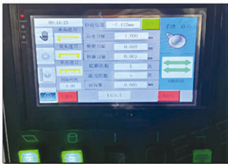
With touch panel, automatic tool dropping. 带触屏操作面板，能自动落刀。
