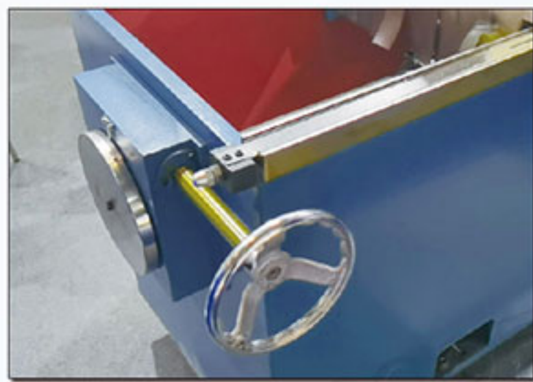
Precise adjustment of electromagnetic sucker angle. 电磁吸盘角度精准调整。
