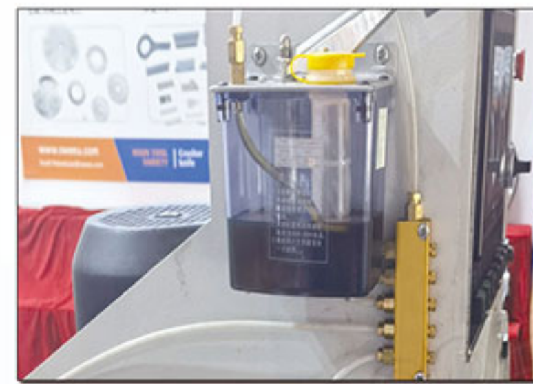
Automatic lubricating pump controlled by Microcomputer. 微电脑控制的自动润滑泵。
