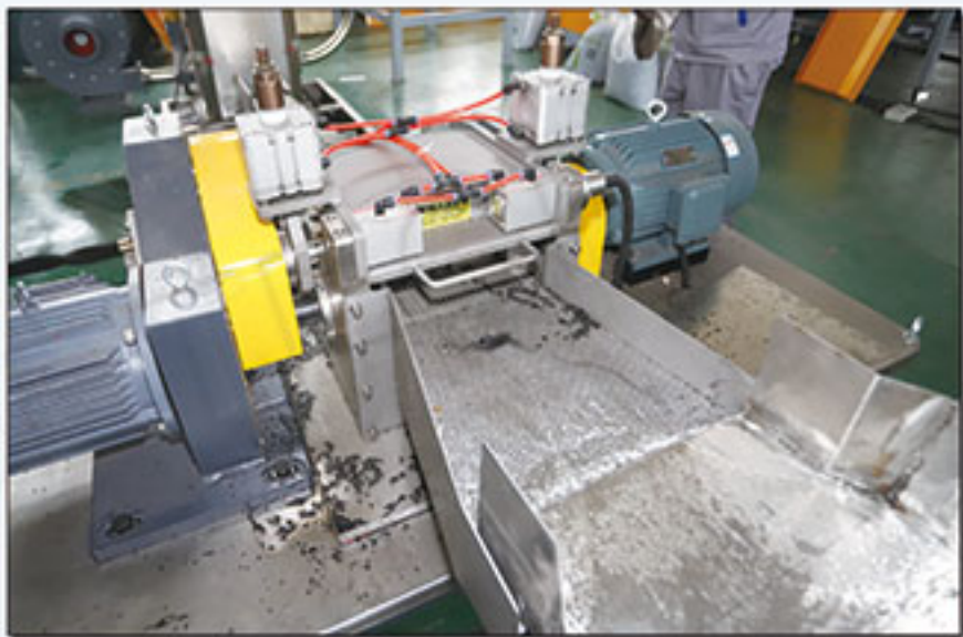
水下切粒系统 Underwater Particle Cutting System The material cools instantly when it enters the water, without sticking to the knife, dragging the wire, or clumping, and the cutting is smooth without blockage. 物料入水瞬间冷却, 不粘刀、不抱丝、不结块, 切粒顺畅无堵料。
