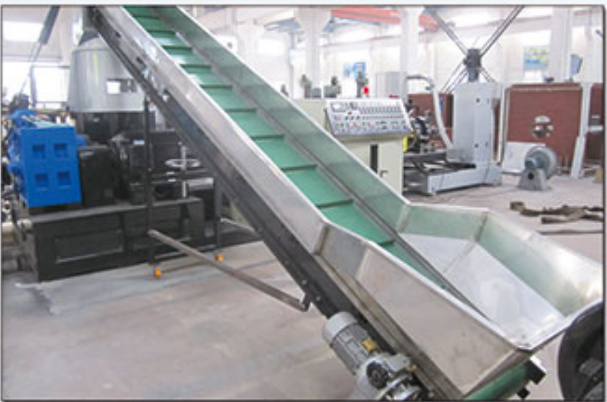
皮带输送 Feeding Plastic material is conveyed into the compactor chamber by belt conveyor, as to rolls films, roller hauling off device is optional device. 原材料由输送带输送到团粒机, 整卷的薄膜牵引装置是可选配置。
