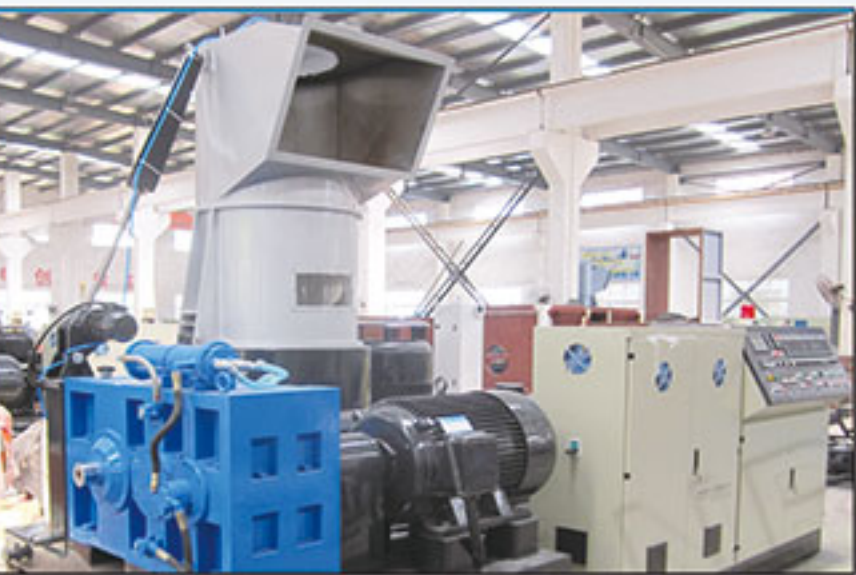
密实仓造粒主机 Extrusion pelletizing system 38CrMoAl screw & barrel nitrogen treatment, double vacuum exhaust, more effectively remove moisture from the material to ensure pellets quality. 38CrMoAl螺杆和机筒氮化处理, 双重真空排气, 更有效地去除物料中的水分, 以确保颗粒质量。
