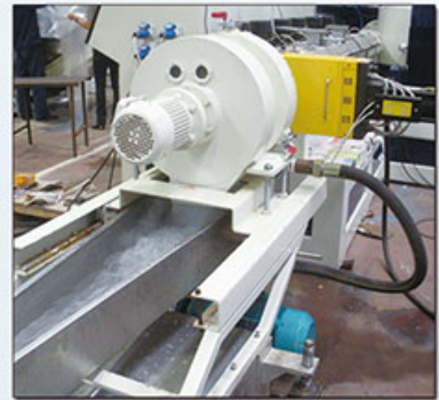
Water ring pelletizer 水环切粒
