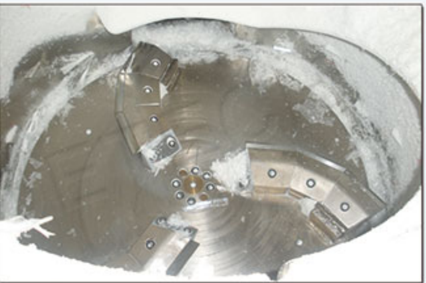
团粒机底座 Agglomerating/Compacting chamber The rotating blades crush the raw material into scraps. Then send it into extruder screw barrel by centrifugal force. 刀片高速转动, 将原材料切成小片, 通过离心力输送到挤出机料筒处。
